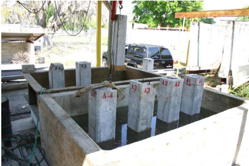
Figure 5.5 View of partially submerged full-size test piles.
